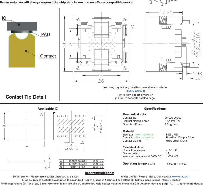
For SMT sockets in general, E-tec recommends the use of locating pegs which can be soldered to the PCB for added mechanical strength.
